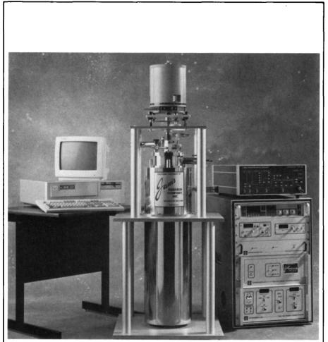
End concerns about accurate data collection with the Janis Research Superconducting Parallel Field Vibrating Sample Magnetometer. This PC compatible, software driven system allows you to preset all parameters, and collect data automatically: magnetization, field and temperature sweep, critical current densities of High Tc materials, hysteresis loop, magnetic moment, etc.
