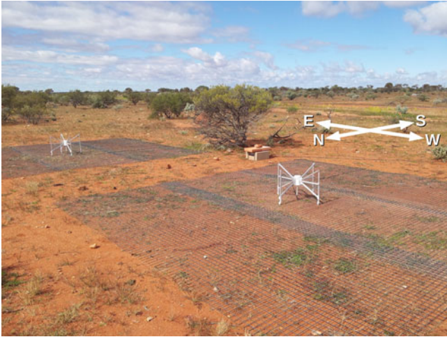
Figure 2. The reference antennas as deployed on site. The RFI-shielded box containing the power and data transfer electronics was protected by bricks, as can be seen near the image centre.
