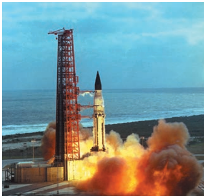
Six liquid hydrogen-fueled engines power the second stage of this Saturn rocket. Courtesy of NASA.
