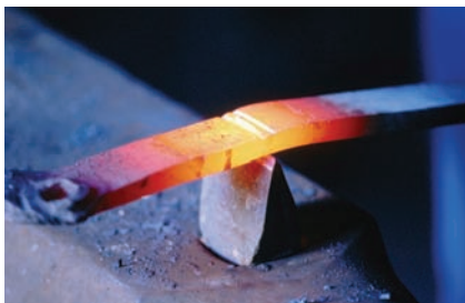
In this iron bar, the highest temperatures occur where the visible radiation is the brightest.
