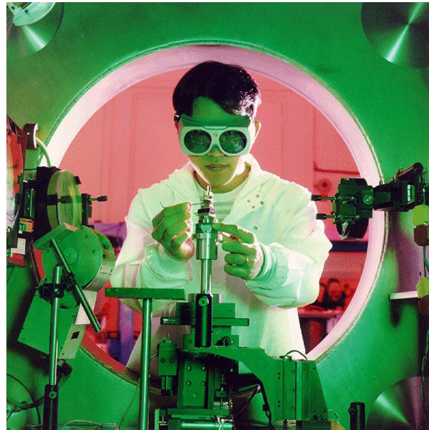
Figure 27. Jiun-Yuan Lin, then at the University of Essex, adjusts an X-ray laser target in the VULCAN target chamber circa late-1990s. (Picture courtesy of STFC.)
