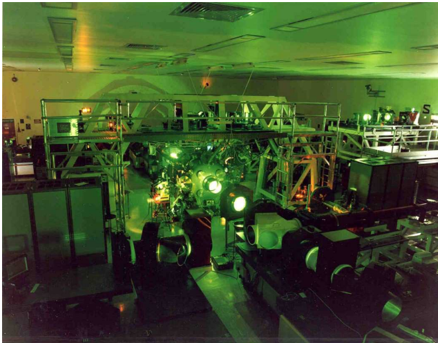
Figure 41. The HELEN target area with self-illumination from the green light produced when the laser beams are frequency doubled. (Picture courtesy of AWE.)
