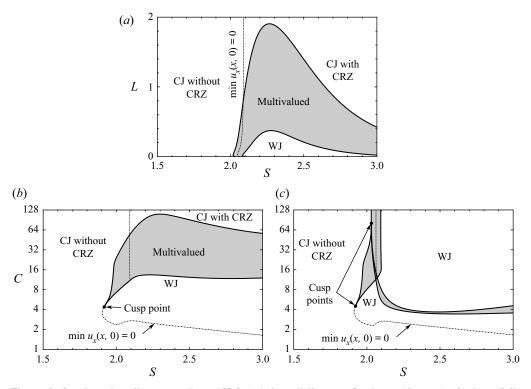
Figure 5. Steady regime diagrams at Re = 150 for (a) the radially unconfined case ( $C \rightarrow \infty$ ), (b) the radially confined case with weak axial confinement (L = 2), and (c) the radially confined case with strong axial confinement (L = 0), where (b,c) are scaled logarithmically in C. Note that instabilities (not indicated) are present over significant portions of the parameter space.
