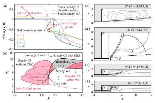
Figure 3. (a) Bifurcation diagrams, (b) stability map scaled logarithmically in C, and (c-f) streamline visualisations illustrating the effect of varying the chamber diameter and swirl ratio with weak axial confinement (L = 2) at Re = 100. All steady solutions are linearly stable unless indicated otherwise.
