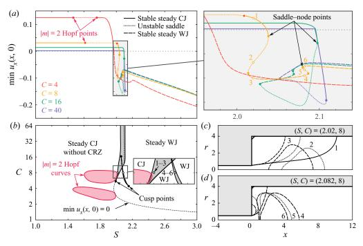
Figure 4. (a) Bifurcation diagrams, (b) stability map scaled logarithmically in C, and (c,d) streamline visualisations illustrating the effect of varying the chamber diameter and swirl ratio with strong axial confinement (L = 0) at Re = 100. All steady solutions are linearly stable unless indicated otherwise.
