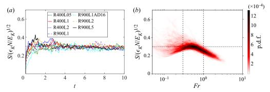
Figure 9. Mean shear rate *S* non-dimensionalized by  $(\epsilon_K N/E_K)^{1/2}$  (*a*) plotted against time *t* for all simulations, horizontal dashed lined indicates empirically observed constant of 0.3, (*b*) presented in the form of a two-dimensional p.d.f. with the turbulent Froude number *Fr*. The p.d.f. is constructed out of the instantaneous data of all simulations within the range of t > 1 and  $0.2 \le z \le 0.8$ . Vertical dashed lines indicate Fr = 0.3 and Fr = 1.
