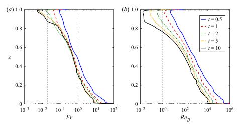
Figure 2. Evolution in time of key local parameters as a function of z for case R900L2. (a) Turbulent Froude number Fr, vertical dotted lines left to right represent Fr = 0.02 (as the upper limit for the strongly stratified regime outlined in Lindborg 2006) and Fr = 1; (b) buoyancy Reynolds number  $Re_B$ , vertical dotted line represents  $Re_B = 1$ .
