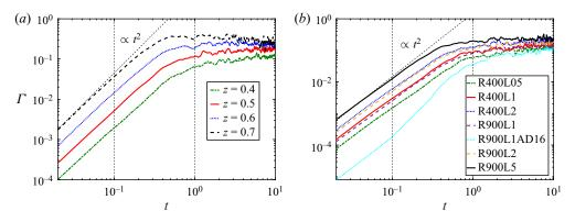
Figure 4. Mixing coefficient  $\Gamma$  plotted against non-dimensional time t (a) at varying vertical locations for case R900L2 (b) at a vertical location of z = 0.5 for all simulations. Vertical dashed lines in both figures represent t = 0.1 and t = 1; the diagonal dashed line represents a line proportional to  $t^2$ .
