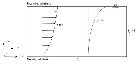
Figure 1. Schematic diagram of the flow configuration; the domain is periodic in x and y.
