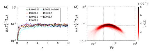
Figure 5. Buoyancy flux *B* normalized by  $E_K^{3/2}/L_N$ , (*a*) as a function of time *t* for all simulations at a vertical location of z = 0.5, (*b*) as a function of the turbulent Froude number *Fr* presented as a two-dimensional probability density function (p.d.f.) for t > 1 and  $0.2 \le z \le 0.8$ . Vertical dashed lines indicate Fr = 0.3 and Fr = 1. Dashed horizontal line in both figures indicates an empirical constant of 0.08.
