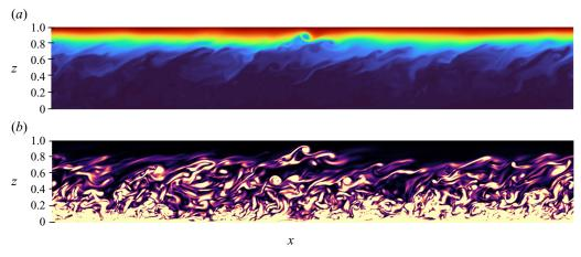
Figure 3. Instantaneous flow visualizations in the vertical (x, z) plane at t = 5 for case R900L2 of (a) the buoyancy field *b* and (b) enstrophy field  $|\omega^2|$ . Flow is moving left to right.
