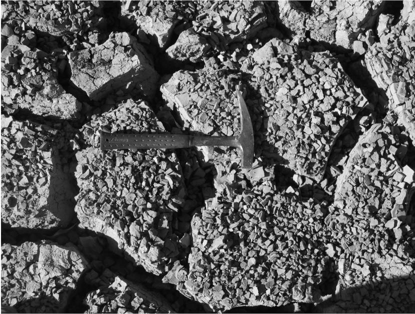
Figure 4.10 Cracking clay soil, Blue Nile Valley, Sudan.
