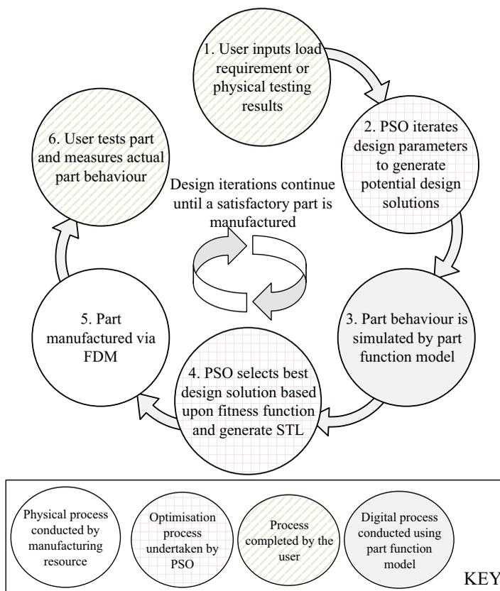
**Figure 6.** Overview of the generative-based design methodology (adapted from Goudswaard *et al.* 2021b).
