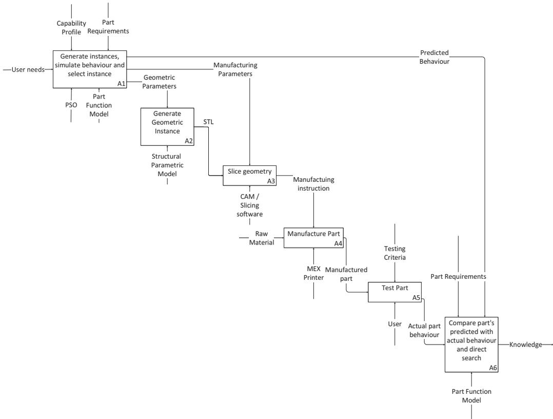
**Figure 7.** IDEF0 activity diagram for single iteration of the GBD methodology.
