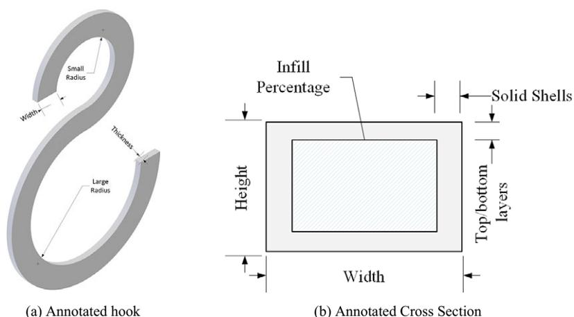
**Figure 8.** Parametrised S-hook and cross-section.
