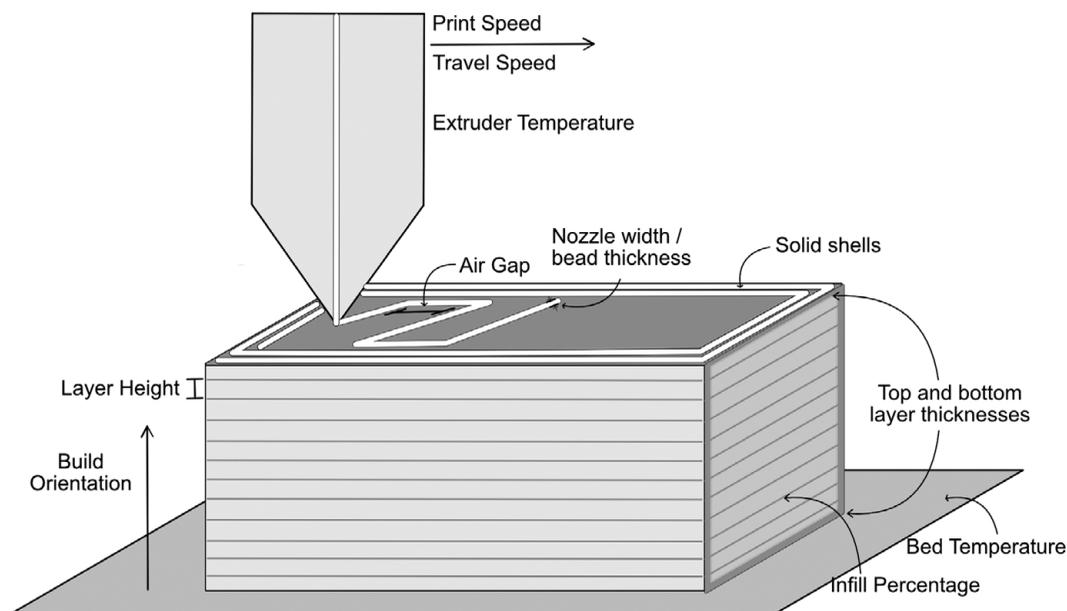
**Figure 2.** MEX manufacturing parameters.
