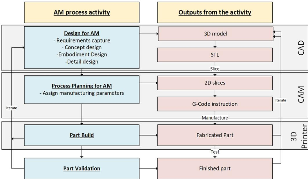
Figure 3. Traditional CAD AM design process stages and respective outputs. Adapted from Qin *et al.* (2019).
