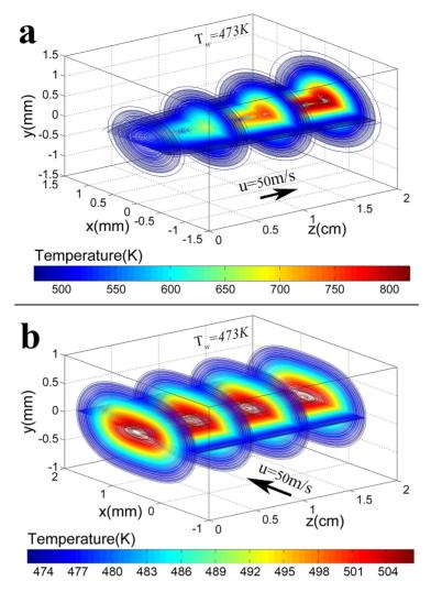
Figure 4. Three-dimensional temperature distribution under different flow directions. The velocity of flow and wall temperature in (a) and (b) are 50 m/s and 473 K.
