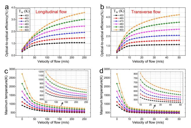
Figure 7. Optical-to-optical efficiency and maximum temperature as a function of flow velocity with different wall temperature at pump intensity of  $5 \times 10^{10}$  W/m<sup>2</sup>.
