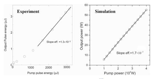
**Figure 3.** Comparison of slope efficiency between experiment<sup>[19]</sup> and simulation results.
