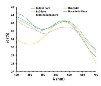
Fig. 2. Reflectance curves for tetrahedrite-(Hg) in air. For comparison, the reflectance curves of type material from Buca della Vena, cotype samples from Jedová hora and Rožňava, and literature data are shown.
