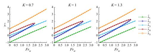
Figure 9. Effect of the earth-pressure coefficient K on the dimensionless eigenvalue trends. Results are obtained considering  $Fr_s/Fr_w = 0.7$ ,  $C_w = 0.5$ ,  $C_e^e = 0.37$  and  $\rho_i/\rho_r = 0.353$ .
