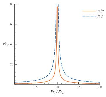
Figure 6. Lower  $(Fr_w^{low})$  and upper  $(Fr_w^{up})$  limits of the non-hyperbolic region as functions of the Froude ratio  $Fr_3/Fr_w$ . Results are obtained, as in figure 4, considering  $C_w = 0.5$ ,  $C_r^e = 0.37$ , K = 1 and  $\rho_i/\rho_r = 0.353$ .
