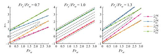
Figure 14. Comparison between the dimensionless eigenvalues of the PI-RIW model and the approximated eigenvalues used by Pudasaini & Krautblatter (2014) to solve their TPPK model. Parameters used in these plots are the same used in figure 5. The TPPK eigenvalues are marked by continuous lines with symbols, while those of the PI-RIW model are denoted by dashed lines without any type of distinction (see figure 5 for details in the PI-RIW eigenvalues).
