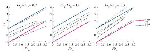
Figure 13. Comparison between the dimensionless eigenvalues of the MP-RIW and of the PI-RIW models. Parameters used in these plots are the same used in figure 5. The MP-RIW eigenvalues are marked by continuous lines with symbols, while those of the PI-RIW model are denoted by dashed lines without any type of distinction (see figure 5 for details in the PI-RIW eigenvalues).
