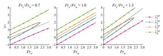
Figure 11. Comparison between the dimensionless eigenvalues of the TP-RIW and of the PI-RIW models. Parameters used in these plots are the same used in figure 5. The TP-RIW eigenvalues are marked by continuous lines with symbols, while those of the PI-RIW model are denoted by dashed lines without any type of distinction (see figure 5 for details in the PI-RIW eigenvalues).
