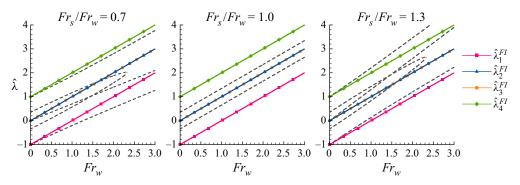
Figure 10. Comparison between the dimensionless eigenvalues of the FI-RIW and of the PI-RIW models. Parameters used in these plots are the same used in figure 5. The FI-RIW eigenvalues are marked by continuous lines with symbols, while those of the PI-RIW model are denoted by dashed lines without any type of distinction (see figure 5 for details in the PI-RIW eigenvalues).
