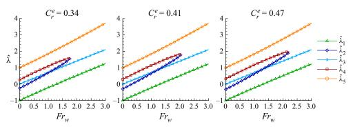
Figure 8. Effect of the rock equivalent concentration  $C_r^e$  on the dimensionless eigenvalue trends. Results are obtained considering  $Fr_s/Fr_w = 0.7$ ,  $C_w = 0.4$ , K = 1 and  $\rho_i/\rho_r = 0.353$ .
