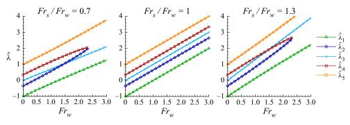
Figure 5. Effect of the Froude ratio on the dimensionless eigenvalue trends. Results are obtained considering  $C_w = 0.5$ ,  $C_r^e = 0.37$ , K = 1 and  $\rho_i/\rho_r = 0.353$ .
