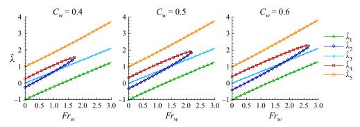
Figure 7. Effect of the water concentration  $C_w$  on the dimensionless eigenvalue trends. Results are obtained considering  $Fr_s/Fr_w = 0.7$ ,  $C_r^e = 0.34$ , K = 1 and  $\rho_i/\rho_r = 0.353$ .
