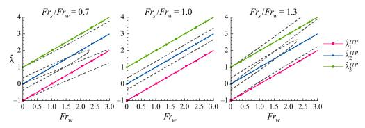
Figure 12. Comparison between the dimensionless eigenvalues of the ITP-RIW and of the PI-RIW models. Parameters used in these plots are the same used in figure 5. The ITP-RIW eigenvalues are marked by continuous lines with symbols, while those of the PI-RIW model are denoted by dashed lines without any type of distinction (see figure 5 for details in the PI-RIW eigenvalues).
