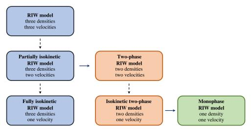
Figure 1. Classes of simplified models obtained from the RIW approach by imposing an isokinetic condition moving in the vertical direction (dashed arrow) and the incompressibility assumption moving in the horizontal direction (continuous arrow). The filling colours represent the number of phases considered (blue, three; orange, two; green, one).
