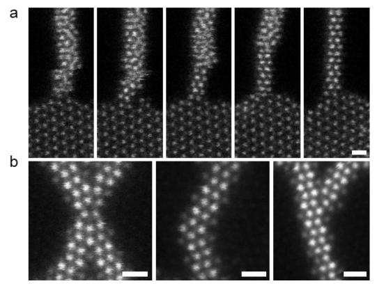
Figure 1: *In-situ* fabrication of nanowires from a TMDC monolayer and different types of junctions. (a) Sequential ADF images showing the fabrication process of an individual MoS nanowire entirely within a semiconducting  $MoS_2$  monolayer. (b) ADF images of different types of nanowires and ramified junctions created by advanced control of the electron irradiation inside the STEM, demonstrating the diversity of building blocks made from these nanowires. Scale bars: 0.5 nm.
