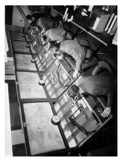
by flight-progress strips indicating time and altitude over each designated reporting point. The controller maintains altitude or time separation through each reporting point. The a.t.c. centre depicted is Uxbridge (transferred to London Flight-progress boards—the basis of present-day separation between aircraft by air traffic control. Flight plans are represented Airport in 1954 on being integrated with Southern Radar).
