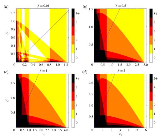
FIGURE 2. (Colour online) Linear stability regions for  $\gamma = 2$  and a range of Reynolds numbers. The number of unstable modes within regions in the  $\nu_1 - \nu_2$  plane is displayed, where we have only counted the pairs or quartets of modes as one. The diagonal lines correspond to  $\nu_1 = \nu_2$  along which we perform numerical simulations.
