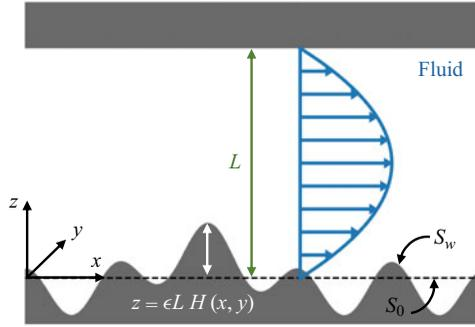
Figure 1. Sketch of pressure-driven flow between the lower corrugated surface  $S_w$  and the upper planar wall (side view). Here,  $L$  denotes the distance between the upper surface and a reference surface  $S_0$  at  $z = 0$ ,  $H(x, y)$  is the shape function, and  $\epsilon$  is the surface roughness.
