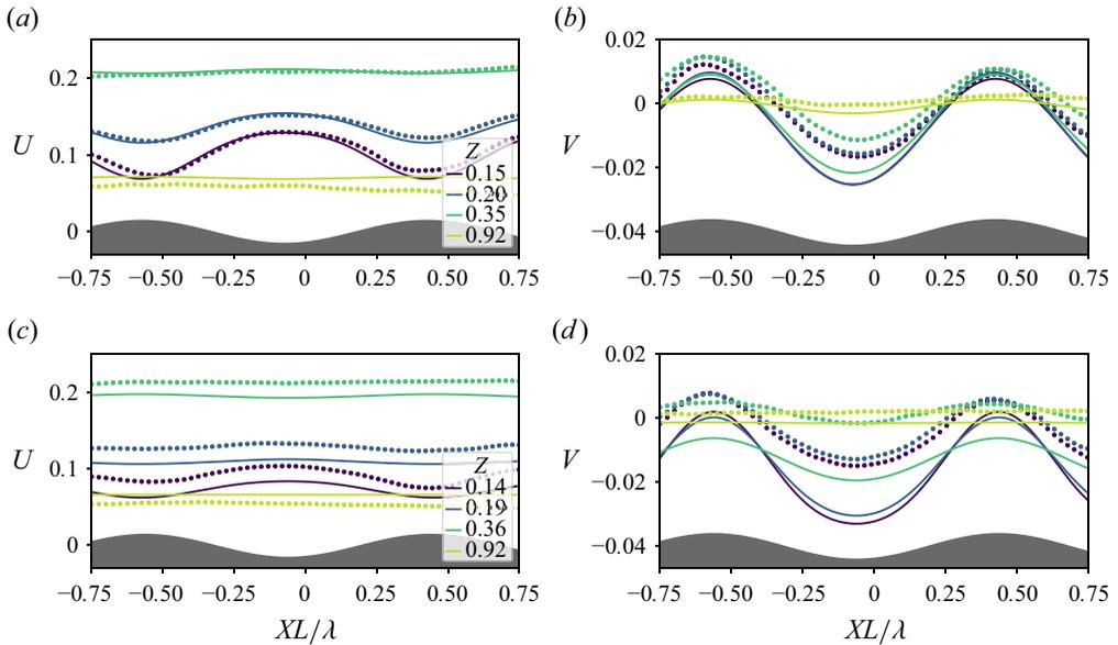
Figure 5. Theoretical and experimental velocities for varying  $\lambda/L$ . The measured experimental and theoretical  $X$  and  $Y$  velocities,  $U$  and  $V$ , along  $Y = 0$  for (a,b)  $\lambda/L = 1.87$  and (c,d)  $\lambda/L = 0.98$  for varying  $Z$ -positions. The symbols indicate the experimental data, and the solid lines are the theoretical prediction. The grey areas indicate the surface shape at the position along  $X$ .
