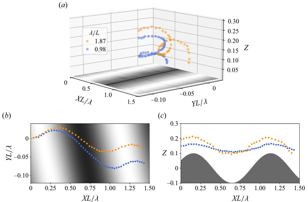
Figure 7. Three-dimensional experimental helical trajectories of tracer particles. (a) Three-dimensional particle trajectories over  $1.5\lambda$  for  $\lambda/L = 1.87$  and  $0.98$  (see experimental methods in § 3). (b) Projection of the three-dimensional trajectories onto the  $XY$ -plane. (c) Projection of the three-dimensional trajectories onto the  $XZ$ -plane.
