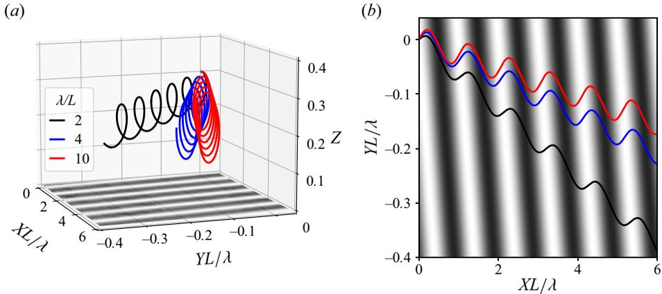
Figure 8. Three-dimensional theoretical helical trajectories of neutrally buoyant point-particles. (a) Three-dimensional particle trajectories over  $6\lambda$  for  $\lambda/L = 2, 4$  and  $10$ . (b) Projection of the three-dimensional trajectories to the  $XY$ -plane. Here,  $Z(0) = 0.3$  for all trajectories.
