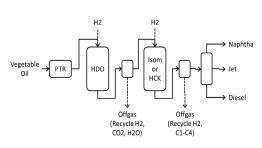
Figure 4. Schematic of representative HVO Plant.
