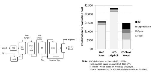
Figure 7. Schematic of representative FT-diesel plant. Figure 8. Production cost structures of hydrogenated vegetable oil, hydrogenated algal oil and FT-diesel.
