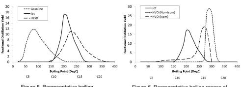
Figure 5. Representative boiling ranges of fossil gasoline, jet and diesel.
