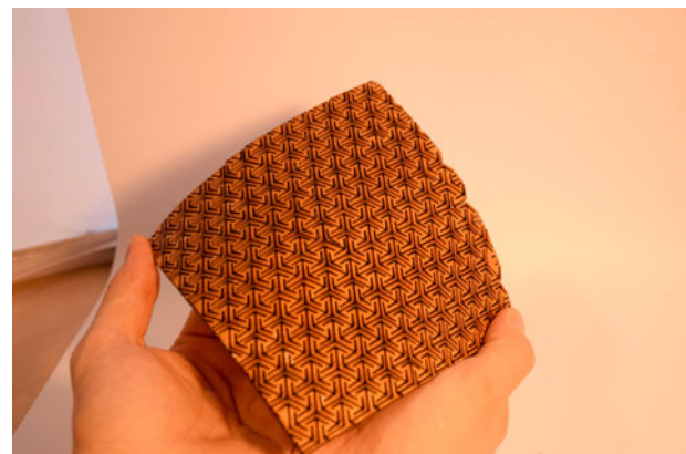
Fig. 3. Example of a laser-cut plate used to prototype a shape-changing interface.
