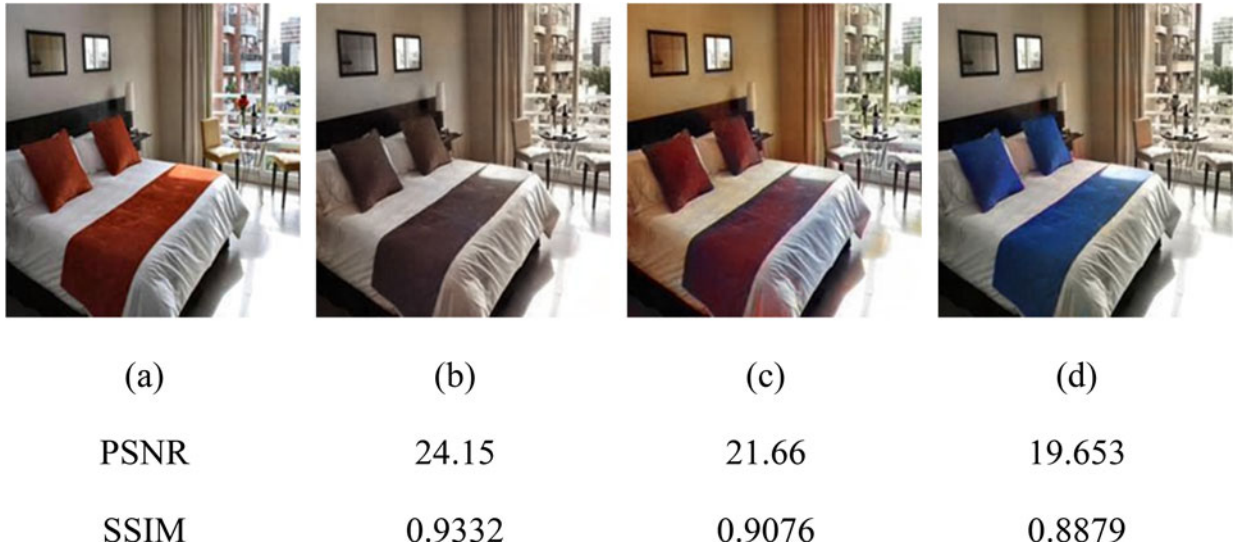
Fig. 5. Problems in using objective image quality assessment metrics to evaluate colorization results. (a) Ground truth. (b) Iizuka et al. [23]. (c) Zhang et al. [25]. (d) Proposed method.
