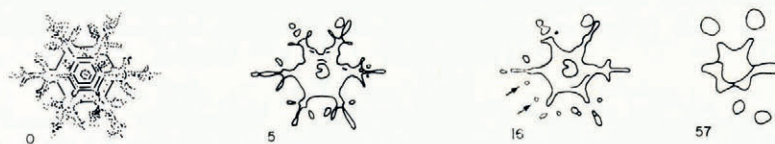
Fig. 2. The progress of equi-temperature metamorphism (the numbers are days). The temperature varied between -2.5^{\circ}\text{C} and -11.5^{\circ}\text{C} . Drawn from photographs in Bader and others (1939).
