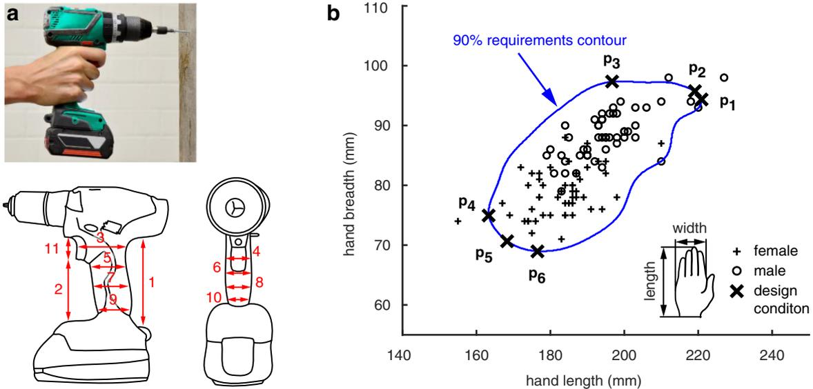
Figure 4. (a) Power tool handle design [adapted from Matthiesen and Germann (2018) with permission from the authors]. The numbers refer to the geometric parameters that were analyzed by Matthiesen and Germann (2018). (b) Requirements contour for the handle design of a power tool.
