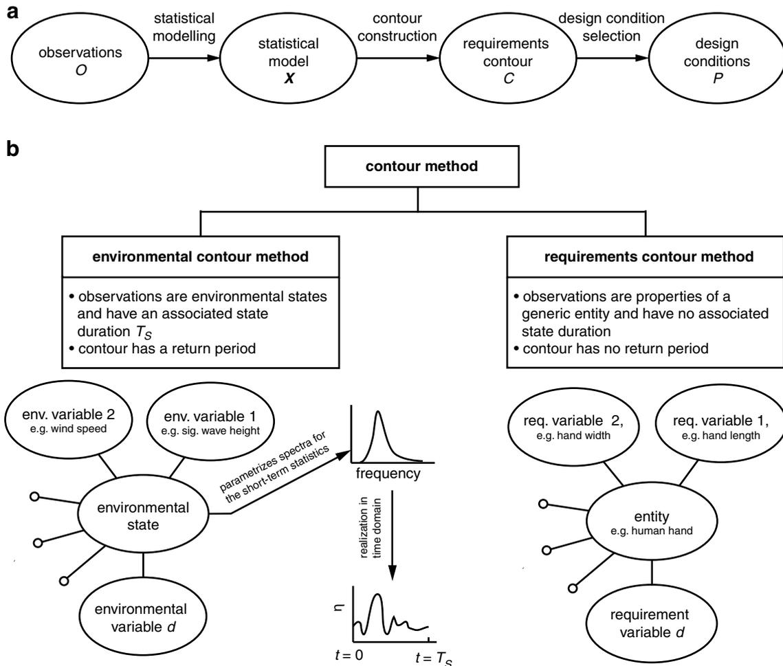
Figure 2. Requirements contour method and its difference to the environmental contour method. (a) In three steps, the requirements contour method maps a sample of properties onto a set of ‘design conditions’. (b) While the environmental contour method is based on time-defined ‘environmental variables’, the requirements contour method deals with ‘requirement variables’, which are time-undefined properties of a common entity.
