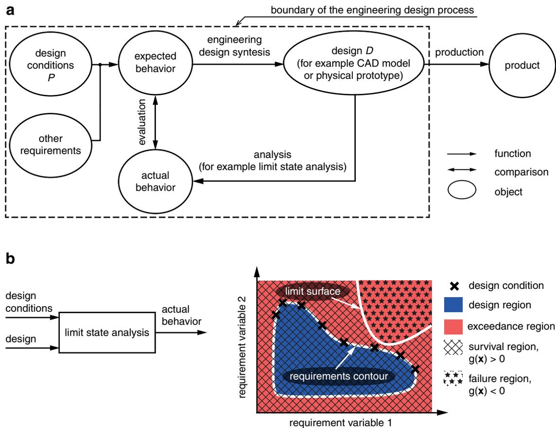
Figure 3. Working with 'design conditions'. (a) Model of the engineering design process and the role that design conditions play in it. Parts of the model's structure are based on Gero (1990). (b) As in structural design, design conditions from a requirements contour can be used in a subsequent limit state analysis. If the failure region does not overlap with the design region the design fulfills the requirement at the specified  $\alpha$ -value.
