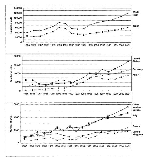
Fig. 1. Installations of industrial robots 1985-1997 and forecast to 2001 and inclusive
