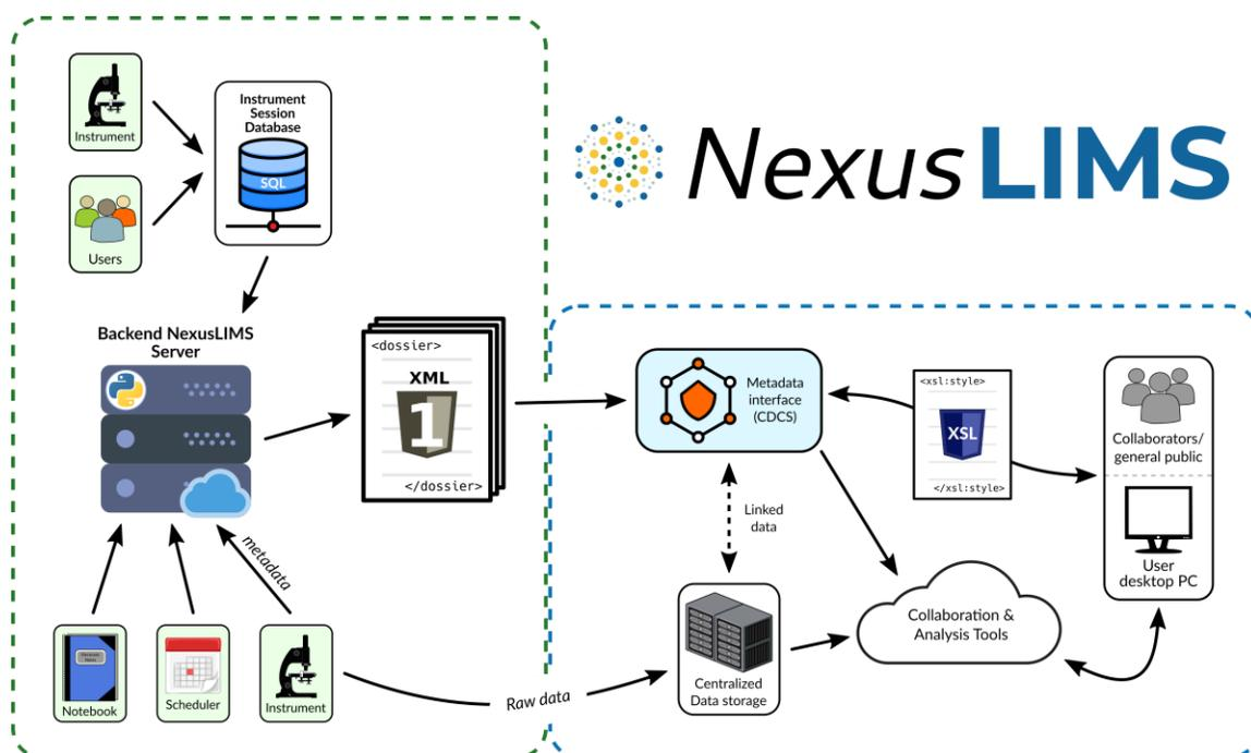
**Figure 1.** A schematic representation of the NexusLIMS system developed at NIST. The “back-end” experimental record building code is depicted on the left, with the “front-end” user-facing interactive portion depicted on the right. See the text for further details. Such a design enables easy access to data from any location via user interaction or API access, and promotes the FAIR principles.
