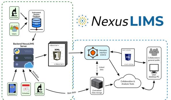
**Figure 1.** A schematic representation of the NexusLIMS system developed at NIST. The "back-end" experimental record building code is depicted on the left, with the "front-end" user-facing interactive portion depicted on the right. See the text for further details. Such a design enables easy access to data from any location via user interaction or API access, and promotes the FAIR principles.
