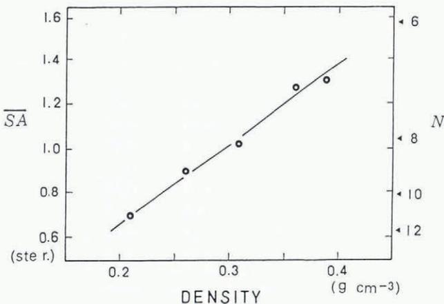
Fig. 7. The mean value of solid angle  $\overline{SA}$  versus snow density.
