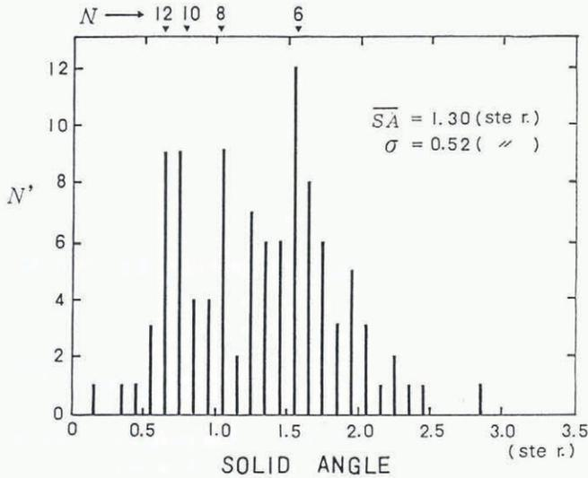
Fig. 6. The distribution of the solid angle of ice bonds (snow density is  $0.39 \text{ g cm}^{-3}$ ).
