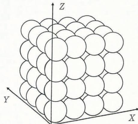
Fig. 1. A perfect packing form of isometric spheres (the cubic lattice,  $N = 6$ ).
