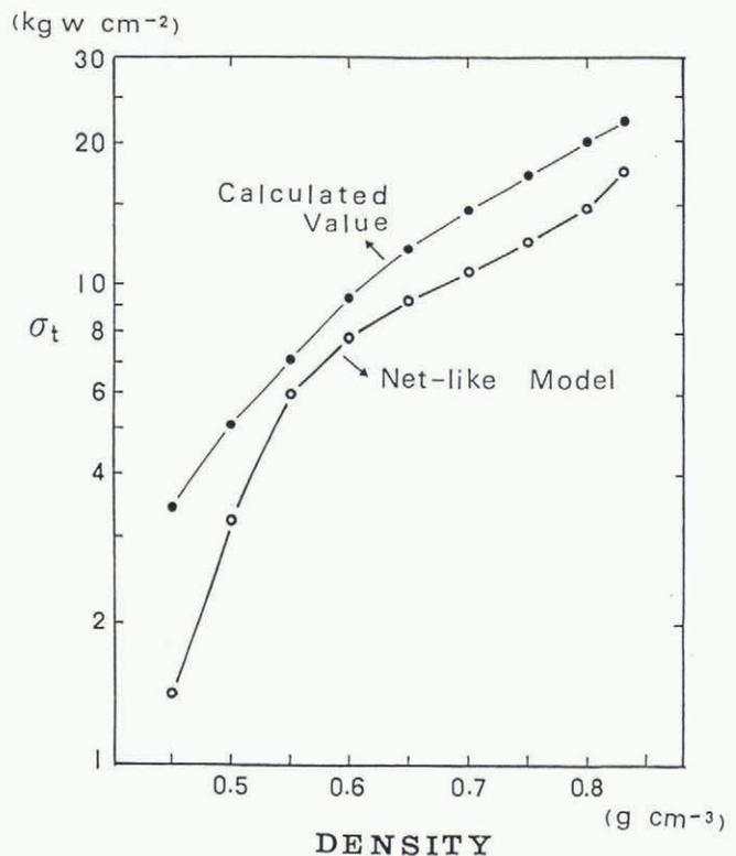
Fig. 9. Comparison of the tensile strength of model with the calculated values for high-density snow.
