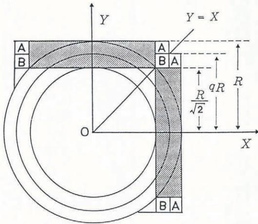
Fig. 4. A sectional view of the model which is composed of crossing branches; the stippled part is the branch of the border model.
