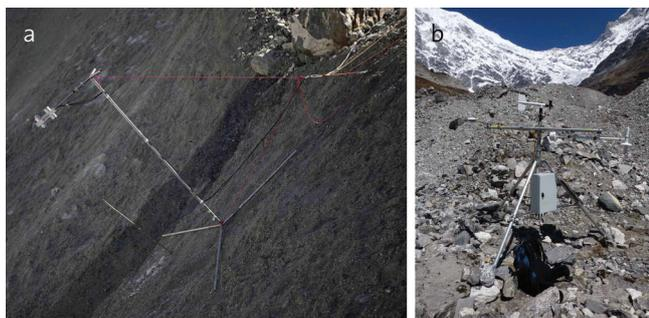
**Fig. 2.** (a) The net-radiometer (Kipp & Zonen CNR1) deployed at the cliff surface at a height of 2 m, measuring incoming and reflected shortwave radiation and incoming and outgoing longwave radiation. (b) The AWS deployed parallel to the debris surface.
