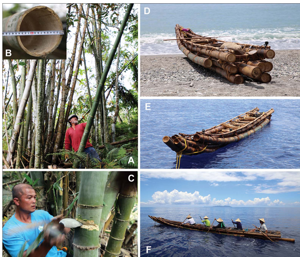
Figure 6. Experiments with the first bamboo raft, IRA 1: A) harvesting of bamboo materials in the coastal mountains; B) cross-section of a D. latiflorus culm; C) experimental cutting of a thick D. latiflorus using replica Palaeolithic stone tools; D) stern of IRA 1; E) bow of IRA 1; F) test at sea (all photographs by Y. Kaifu).
