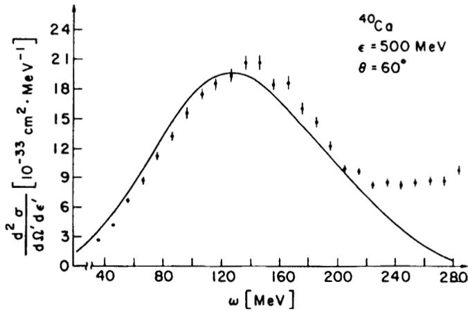
Fig. 21.2. Quasielastic electron scattering from  ${}^{40}_{20}\text{Ca}$  in RMFT compared with experimental values. The calculation assumes a local Fermi gas with the quantities  $m^*(r)$  and  $\rho_B(r)$  taken from a relativistic Thomas–Fermi calculation of these quantities in QHD-I [Ro80, Wa95]. Data are from [Mo71].
