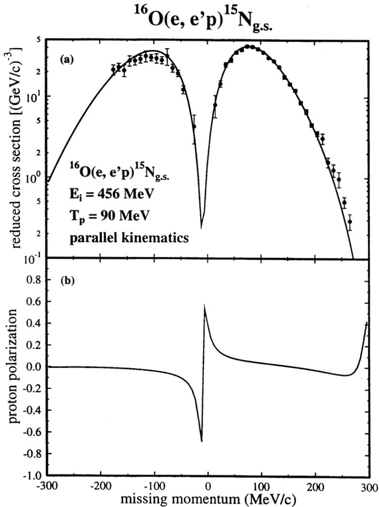
Fig. 21.8. Relativistic Hartree calculation using RIA optical potential and effective current compared with data for  $^{16}\text{O}(e, e'p)^{15}\text{N}_{\text{g.s.}}$  (see text) [He95]. The author is grateful to J. I. Johansson for preparing this figure.
