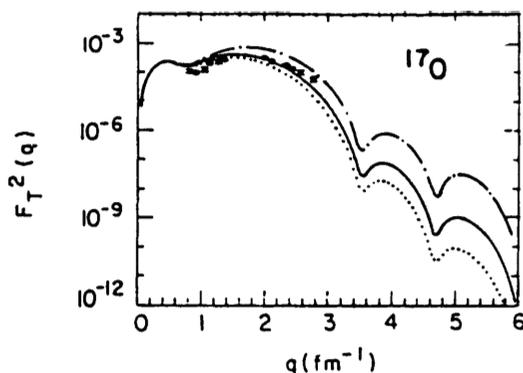
Fig. 21.7. Magnetic form factor squared for  $^{17}_8\text{O}$ . Calculated using relativistic Hartree wave functions and the effective current operator [Ki86, Wa95]. The dotted curve omits the C-M correction factor taken from the harmonic oscillator shell model, and the dashed curve omits the single-nucleon form factor. Data are from [Co65, Mc77, Ar78, Ca82].
