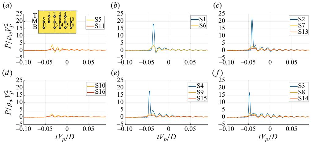
Figure 37. Perturbed tests event *E*: pressure oscillations due to the natural frequency excitation and high aeration.
