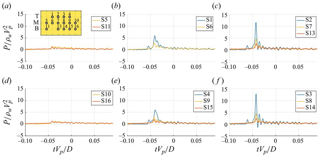
Figure 28. Unperturbed tests event *A*: pressure oscillations due to the natural frequency excitation and low aeration.
