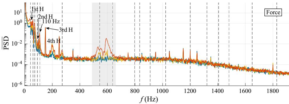
Figure 23. The averaged PSD of slamming force for the perturbed tests for all groups:  $g_1$  in pine green,  $g_2$  in blue,  $g_3$  in yellow,  $g_4$  in red.
