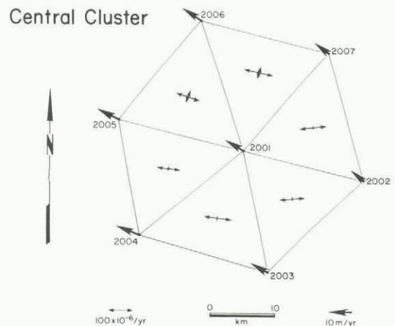
Fig.4. Velocities and strain-rates of the central cluster.
