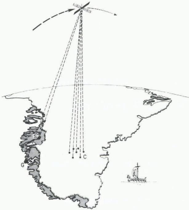
Fig.1. The short-arc method. Locations of stations G (Godthåb) and S (Søndre Strømfjord) are held fixed. Locations of stations C are calculated relative to G and S.
