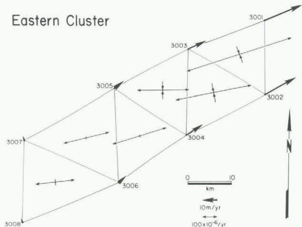
Fig.5. Velocities and strain-rates of the eastern cluster.
