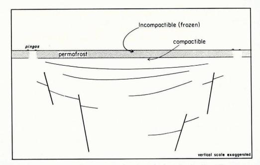
Fig. 2. Development of excess pore pressure beneath permafrost in a region affected by subsidence
