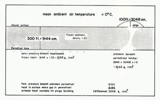
Fig. 3. Artesian head resulting from density difference in a column of frozen sediment and a column of water
