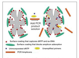
Schematic depiction of differentially functionalized nanoporous particles for purification of polymerase chain reaction products.
