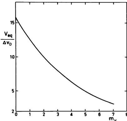
Fig. 1. Doppler shift fluctuations : critical equatorial velocity such that 1 month observing time is requested with a 1 m telescope,  $\lambda / \Delta \lambda = 10^5$ , to reach  $\delta V_{rms} = 10 \text{ cm s}^{-1}$  on a solar type star (we used P. Connes, 1985, estimates of the performances for an optimized absolute accelerometer). The graph gives  $V_{eq} / \Delta v_D$  versus visual magnitude  $m_v$ , with  $\Delta v_D$  = Doppler width of the line.
