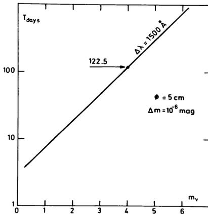
Fig. 3. Exposure time needed to reach a photon-noise of  $10^{-6}$  mag with a device such as shown in Fig. 2, versus the visual magnitude of the star  $m_v$ .
