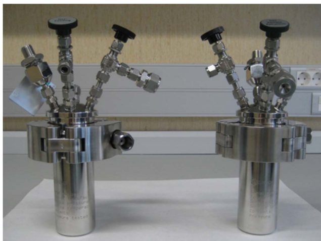
Figure 3 High-pressure steel reactors.
