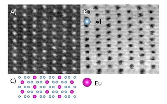
**Figure 1.** A) A HAADF-STEM image of the area of interest that displays no severe scan distortions and was used as a reference image for distortion correction of the 4D-STEM dataset. B) A severely distorted 4DSTEM acquisition with incorrect probe positions. C) An atomic model of EuAl<sub>4</sub> viewed along the [100] zone axis.
