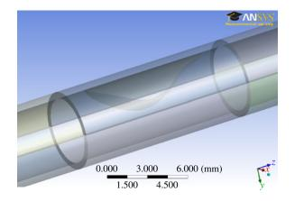
FIGURE 7. Stenosis shape for the 53% growth-updated stenosis model.
