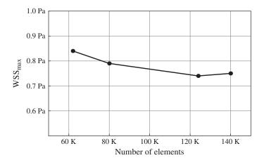
FIGURE 3. Maximum WSS values for four mesh densities.
