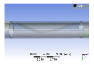
FIGURE 8. Stenosis shape for the 79% growth-updated stenosis model.
