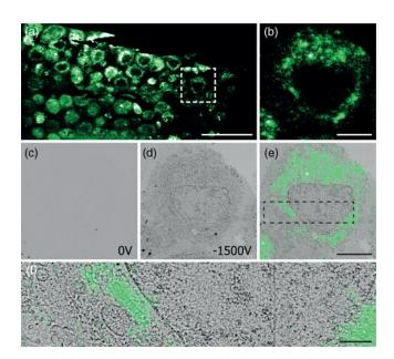
**Fig. 4.** Correlative images of in-resin embedded 100 nm HeLa cell sections labeled with GFP, (**a,b**) FM images in ambient conditions. (**c,d**) EM images using a 1.5 keV landing energy and (**c**) 0 V stage bias and 30  $\mu$ s dwell time, (**d**) –1.5 kV stage bias, and 5  $\mu$ s dwell time. (**e,f**) Manual correlative overlay. Scale bars: (**a**) 50  $\mu$ m, (**b**–e) 10  $\mu$ m, (**f**) 3  $\mu$ m.
