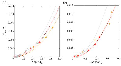
Figure 13. Maximum values of non-dimensional deformation of plates with (a) fixed and (b) free ends.
