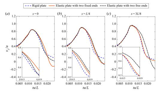
Figure 5. Time history curves of vertical velocity components at the different points locating on a line with z = -0.005L. Plots (a-c) illustrate the results recorded at x = 0, x = L/4 and x = 3L/8. A close-up view of the time history of each vertical velocity component over 0.012 < tu/L < 0.019 is shown in the insets.
