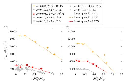
Figure 14. Maximum dimensionless equivalent stress of plates with (a) fixed and (b) free ends.
