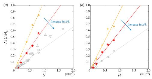
Figure 10. The first crest of momentum, arising in plates with (a) fixed and (b) free ends, just after impact, as a function of the dimensionless impact speed.
