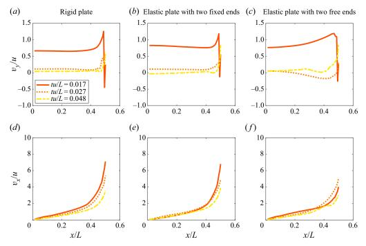
Figure 6. Curves showing distribution of (a-c) vertical and (d-f) horizontal velocity components along a horizontal line located at z = -0.005L. (a,d) Results corresponding to the rigid plate; (b,e) results corresponding to the elastic plate with fixed ends; (c,f) results corresponding to the elastic plate with free ends.
