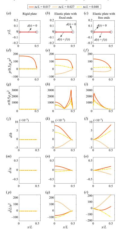
Figure 4. Curves showing the distributions of (d-f) pressure, (g-i) dimensionless equivalent stress, (j-l) dimensionless deformation, (m-o) dimensionless vertical speed, and (p-r) dimensionless vertical acceleration, along plates entering water (a-c).
