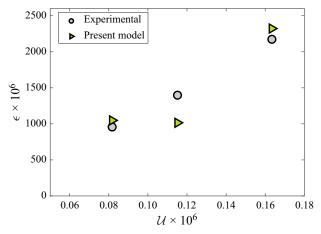
Figure 19. Maximum stain at the middle point of a steel plate entering water at different impact speeds. Circle and triangle markers respectively display experimental and numerical data. Experimental data are taken from Kvalsvold & Faltinsen (1995).
