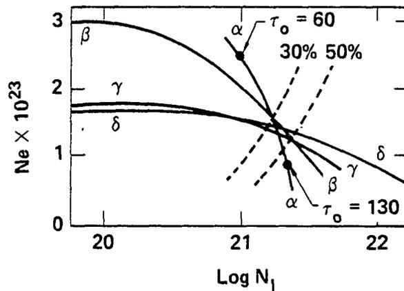
Fig. 3 Example of interpreting x-ray line broadening data to find imploded core densities. Ar-broadened Lyman series lines are fit to various electron densities,  $N_e$ , and ion densities,  $N_i$ . The intersection of the different curves determine the imploded core density. The dashed lines show the curves for when 30% and 50% of the total ion density are in the hydrogen-like ground state.
