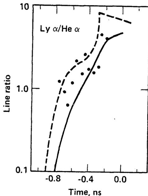
Fig. 2 Example of the time-resolved  $\text{Ly}\alpha/\text{He}\alpha$  ratio of Sulfur from exploding foils. The solid and dashed curves are the predicted line ratio from a 2-d hydrodynamic code coupled with a dynamic ionization model (—) and a steady-state ionization model (---).
