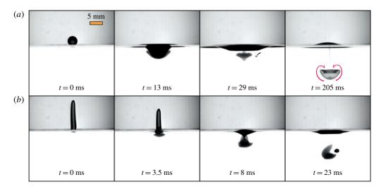
FIGURE 9. (Colour online) Impact of (a) a soft gel droplet ( $\tau_0 = 2$  Pa) at  $U_0 = 0.32$  m s<sup>-1</sup> and (b) a hard gel ( $\tau_0 = 35$  Pa) at  $U_0 = 0.65$  m s<sup>-1</sup>.
