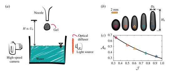
FIGURE 2. (Colour online) (a) Experimental set-up for the investigation of viscoplastic water entry. The shown dimensions are not to scale. (b) Shape of the droplets before impact for different gels (symbols are the same as in figure 1). (c) Variation of the aspect ratio versus  $\mathcal{J} = \tau_0 D_s / \sigma$ . The solid line is an empirical fit of  $\mathcal{A}_0 = \mathrm{e}^{-1.25 \mathcal{J}}$ .
