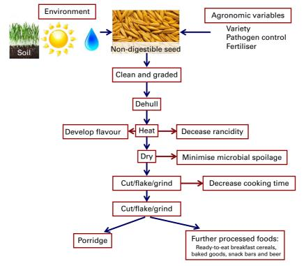
Fig. 1. A flow diagram showing the production of oats on the farm through typical oat-processing operations and production of human foods. The impact of processing operations on the farm variables is included in other sections in this special addition. How the quality of the oats is affected by some processing steps are included in the side boxes. A colour version of this figure can be found online at http://www.journals.cambridge.org/bjn
