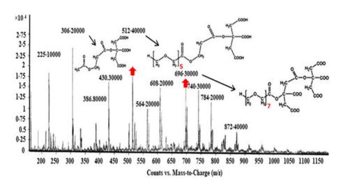
LC-MS was used to confirm the nanodendrimer G2 (Fig. 3). The peaks at 512 and 696 mz-1 in the figure represent 5 and 7 repeating units (CH2-O-CH2, Mw = 44) of PEG with a citric acid group, respectively.
