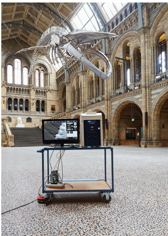
Figure 3: The Hitachi TM4000Plus portable electron microscope at Hintze Hall in the National History Museum, London, UK.
