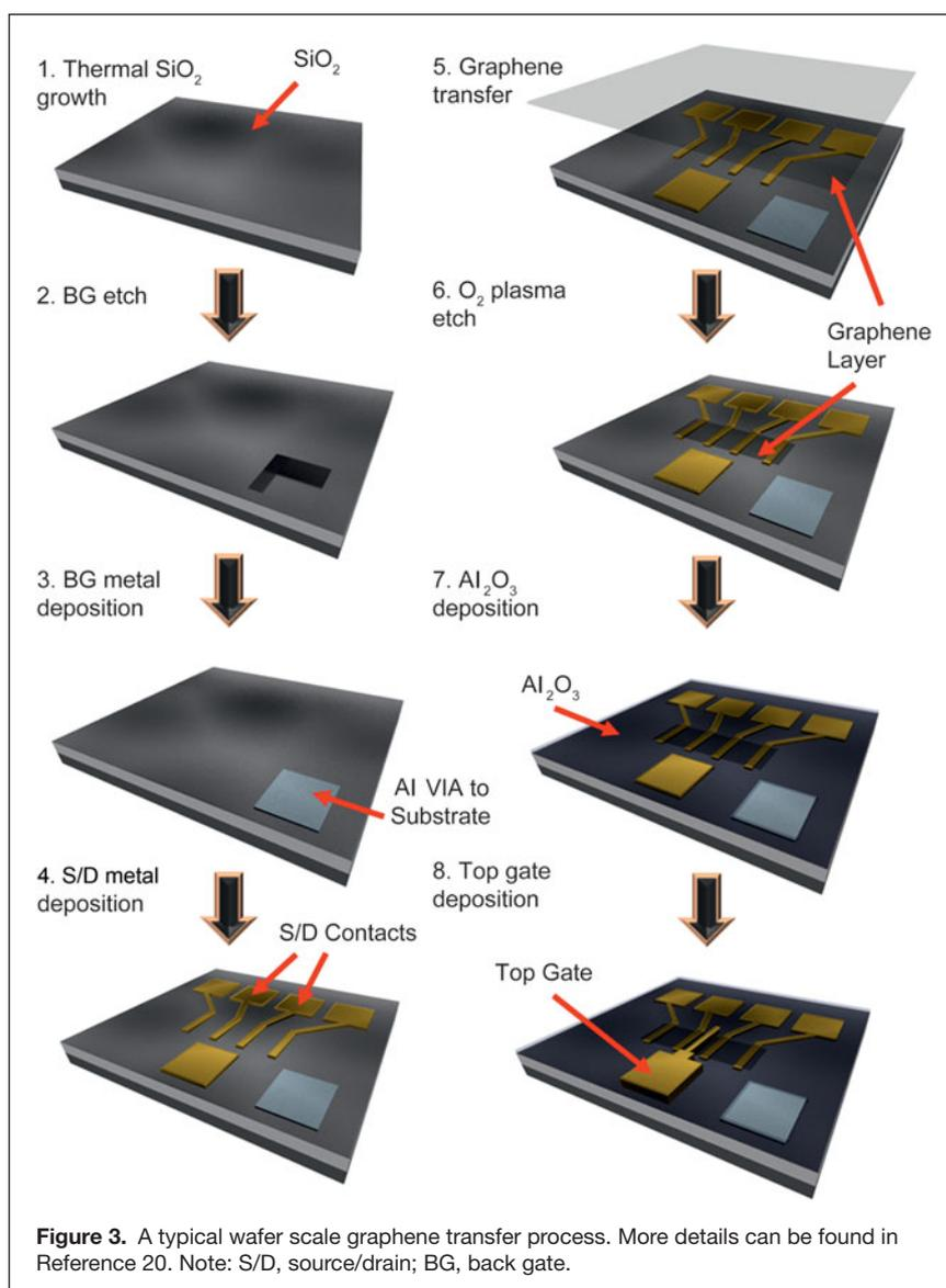
**Figure 3.** A typical wafer scale graphene transfer process. More details can be found in Reference 20. Note: S/D, source/drain; BG, back gate.
