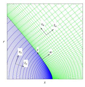
Figure 14. Orthogonal and surface reference frames defined near the meniscus tip.
