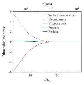
Figure 5. Components of the normal stress on the surface of the meniscus for  $\Phi_E = 1900 \text{ V}$  and  $\Delta G_S = 1.7 \text{ eV} (L_c = 2.77 \text{ nm}).$
