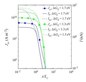
Figure 7. Emitted current density  $J_{\omega}$ , total emitted current  $I_{I}$ , and estimated total current for an equipotential meniscus  $I_{I\sigma}$ , for  $\Phi_{E}=1900 \text{ V}$  and two values of the ion solvation energy.
