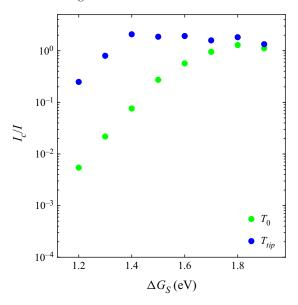
Figure 13. Ratio between the emitted current derived from scaling law (4.3) and the current computed with the simulations, for  $\Phi_E = 1900 \text{ V}$ . The scaling law is evaluated with the upstream temperature (green), and with the temperature at the tip of the meniscus (blue).
