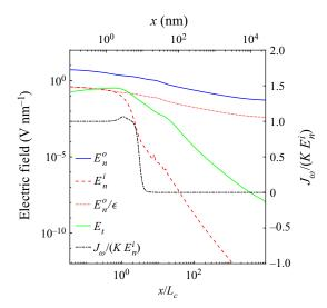
Figure 6. Components of the electric fields and ratio  $J_{\omega}/KE_n^i$  on the surface of the meniscus, for  $\Phi_E=1900~{\rm V}$  and  $\Delta G_S=1.7~{\rm eV}~(L_c=2.77~{\rm nm}).$
