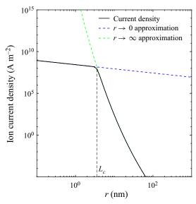
Figure 2. Estimation of the ion current density emitted from a Taylor cone, (2.20), computed with T = 25 °C,  $\varepsilon = 10$ ,  $\Delta G_S = 1.6$  eV,  $\gamma = 0.05$  N m<sup>-1</sup> and K = 1 S m<sup>-1</sup>.
