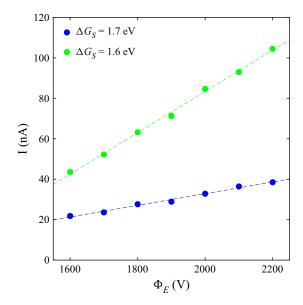
Figure 10. Emitted ion current vs emitter potential for two values of the solvation energy.
