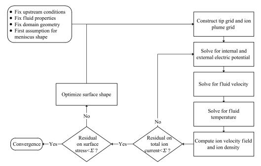
Figure 3. Flow chart of the algorithm for solving the system of equations.
