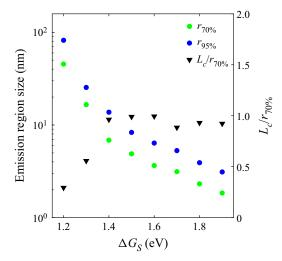
Figure 12. Radius of the emission region from which 70 % and 95 % of the ion current is emitted, and ratio between the characteristic length of the emission region and the computed value.
