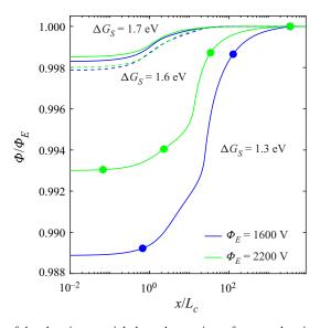
Figure 8. Variation of the electric potential along the meniscus for several emitter potentials and ion solvation energies.
