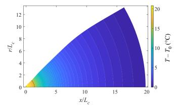
Figure 9. Temperature increase in region 3 for  $\Phi_E = 1900 \text{ V}$  and  $\Delta G_S = 1.7 \text{ eV}$ . The red line marks  $K_n = 0.1$ .
