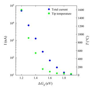
Figure 11. Effect of the ion solvation energy on the current of emitted ions and the tip temperature  $(\Phi_E = 1900 \text{ V})$ .
