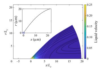
Figure 4. Shape of the meniscus and magnitude of the liquid velocity and streamlines in region 3, for  $\Phi_E = 1900 \text{ V}$  and  $\Delta G_S = 1.7 \text{ eV}$ . The red line marks  $K_n = 0.1$ . The values of the characteristic velocity and length are  $V_{fc} = 4.15 \text{ m s}^{-1}$  and  $L_c = 2.77 \text{ nm}$ .
