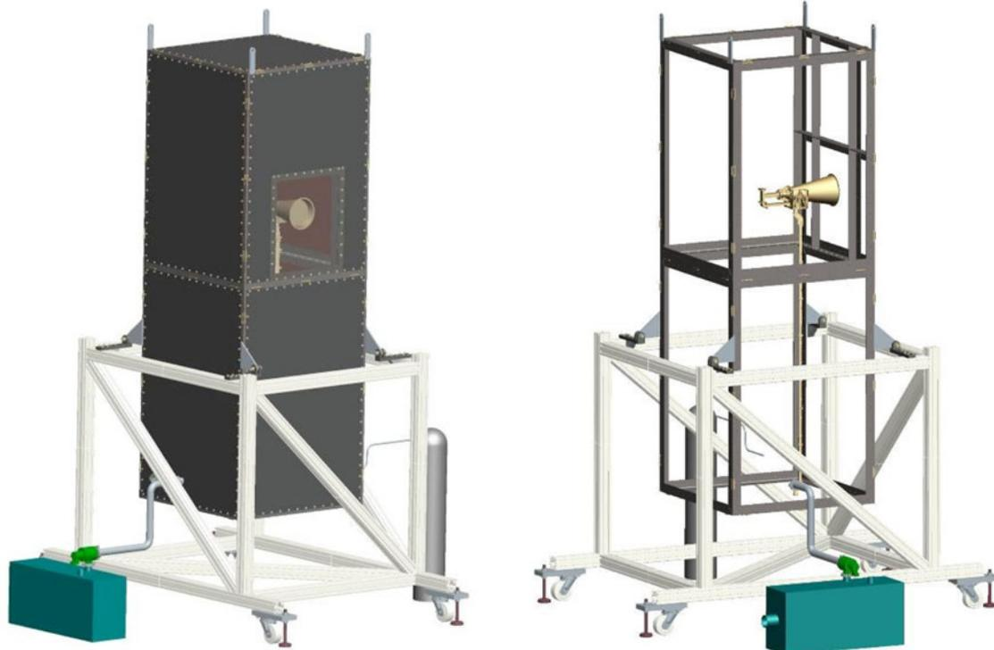
Fig. 4. RF oven overview (left) and its structure with MGA-RFA placement (right).
