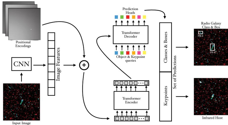
**Figure 3.** An overview of the multimodal modelling strategy introduced in this study. In the context of the Gal-DETR model (refer to Section 3.1), we introduce a keypoint estimation module within the transformer encoder-decoder framework. This enables the simultaneous detection of categories and bounding boxes for radio galaxies, and the positions of infrared hosts. A similar multimodal strategy is introduced for Gal-Deformable DETR and Gal-DINO (as detailed in Sections 3.2 and 3.3).
