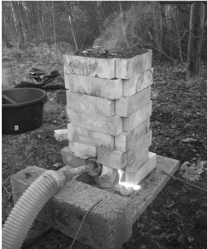
Figure 1 Furnace used in the iron smelting experiment. The furnace is constructed with light-gravel blocks surrounded by firebricks. A blower supplies air into the process. In the figure, the molten slag is draining out from the process via an opening at the lower right-hand side of the furnace.
