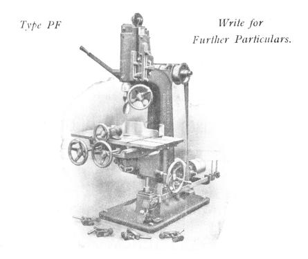
For boring, drilling, and recessing the bosses of propellers, etc.; half lapping the laminations; recessing and drilling the spars, etc.
