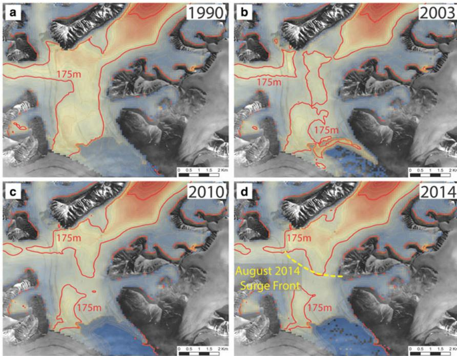
**Fig. 10.** Thinning of the glacier from 1990 to 2014, showing the 175 m thickness contour which delimits the area of potential bed freezing. The 2003 map was derived by extrapolation back from the 2010 image, using measured changes in ice thickness.
